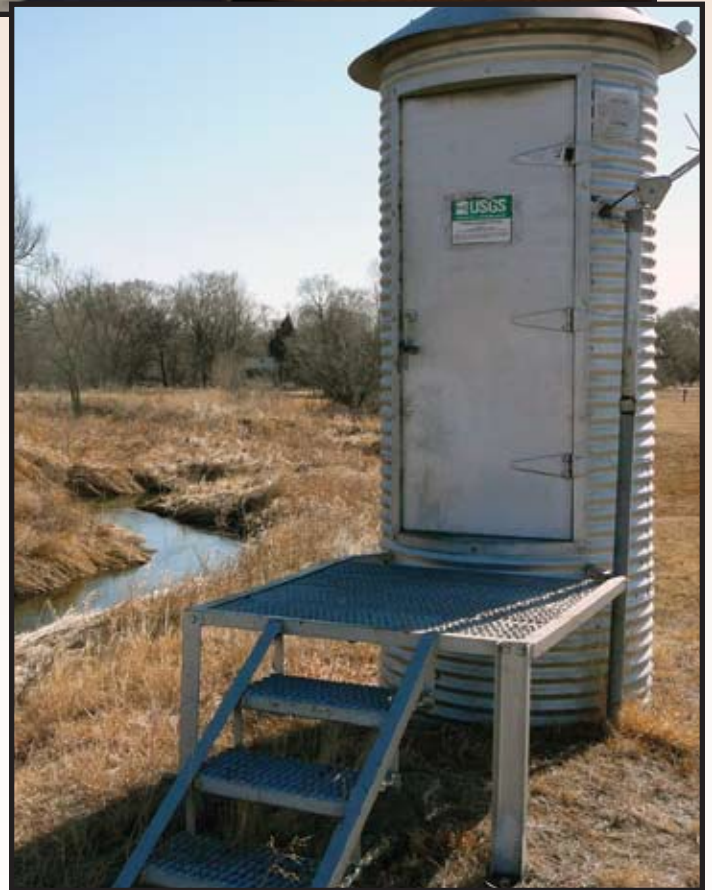
A U.S. Geological Survey stream flow gauge on Rock Creek in southwest Nebraska will measure increased flows expected from the augmentation project.
